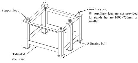
2 Install the Graplate on the dedicated steel stand using a block and tackle or other lifting machinery.
